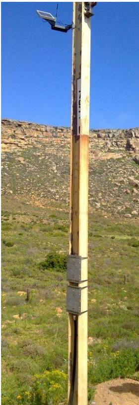
Fig. 15. Data logger, wireless modem and solar panel installation.
