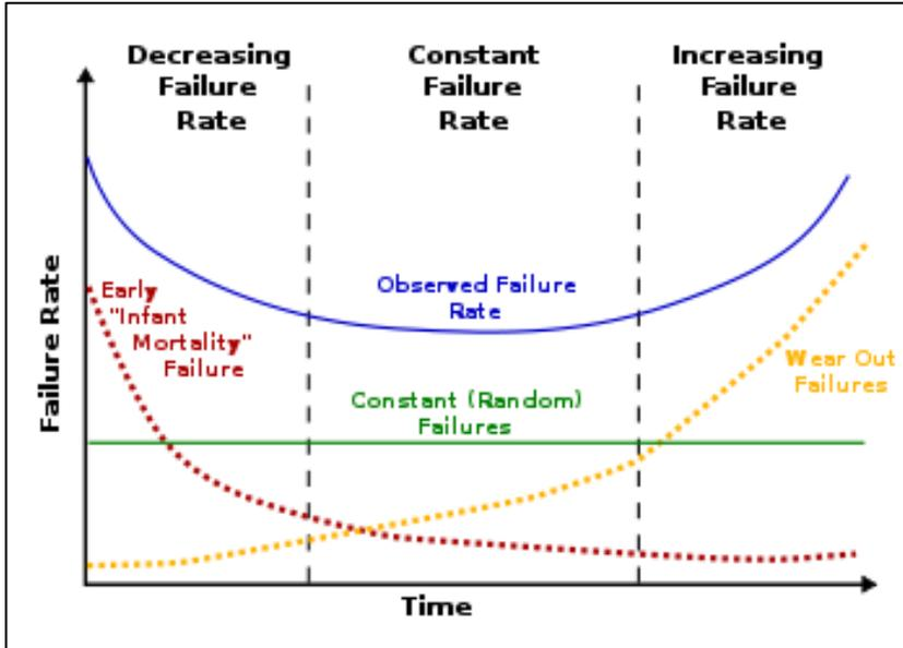
Fig. 1. The bathtub curve hazard function.
