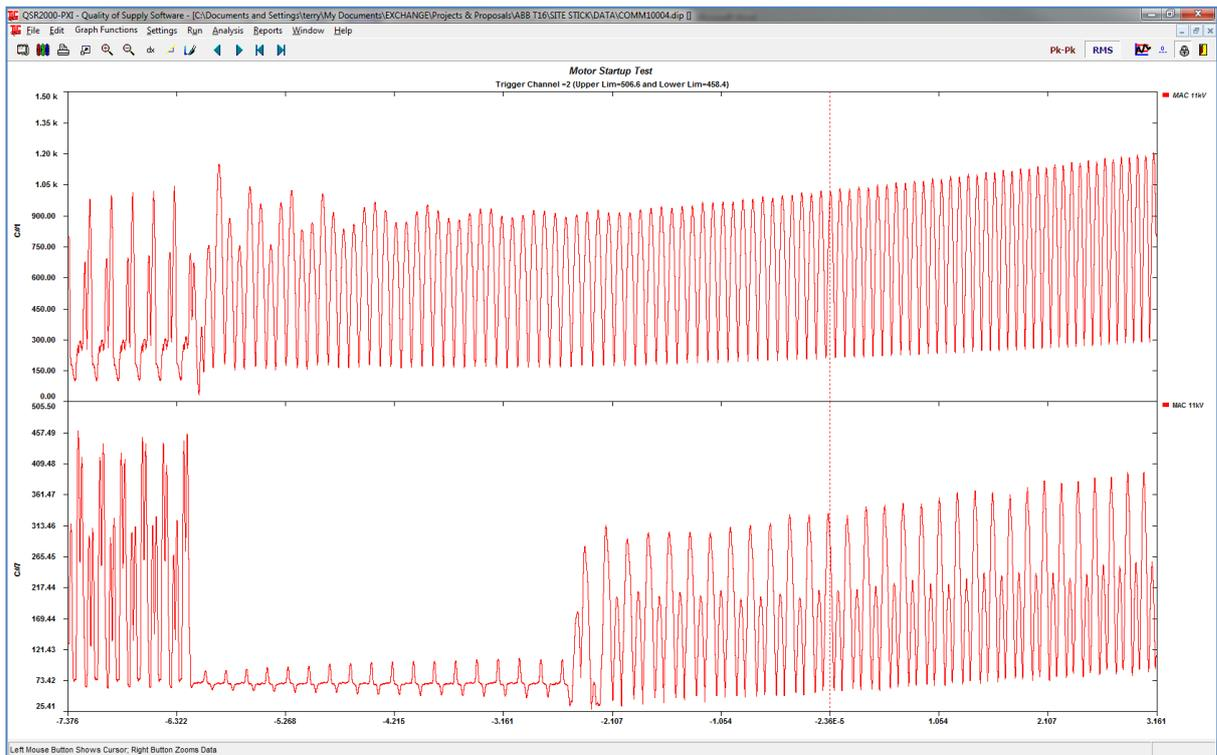
Fig. 6. LCI waveforms from initial starting of the motor.
