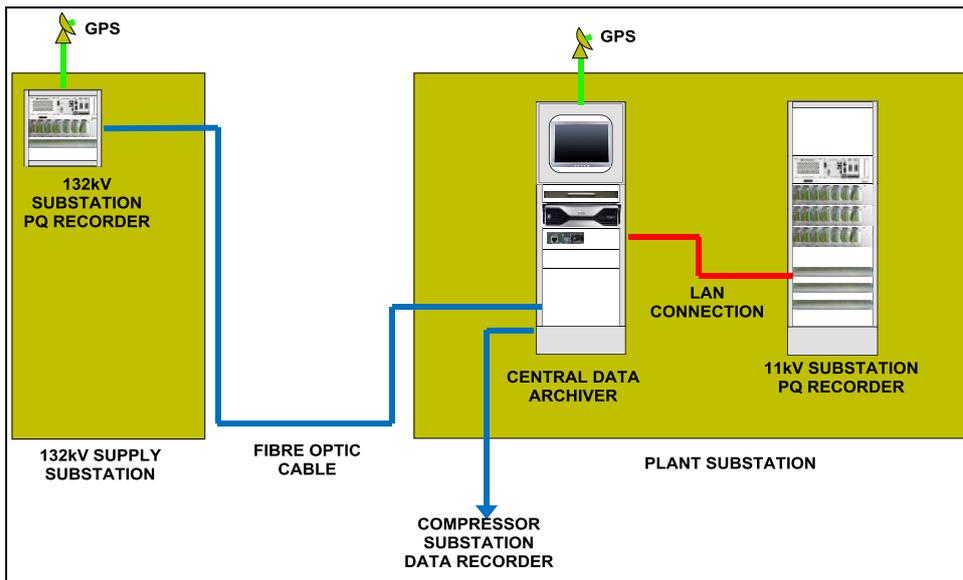
Fig. 3. Block diagram of compressor drive monitoring system.
