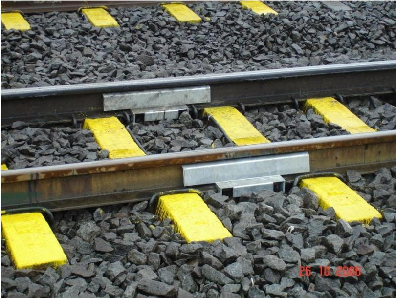
Fig. 14. Track mounted rail stress and temperature sensor.
