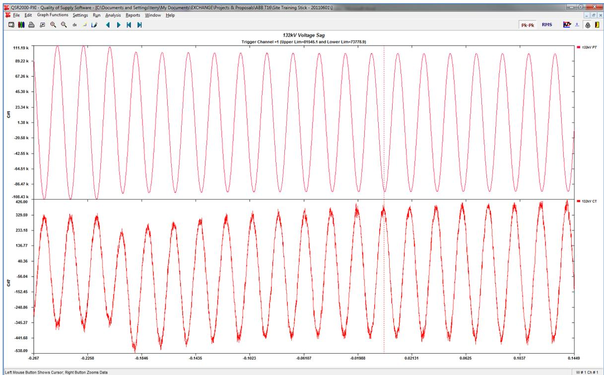
Fig. 9. Supply current waveform to the drive during a dip on 132kV substation supply.
