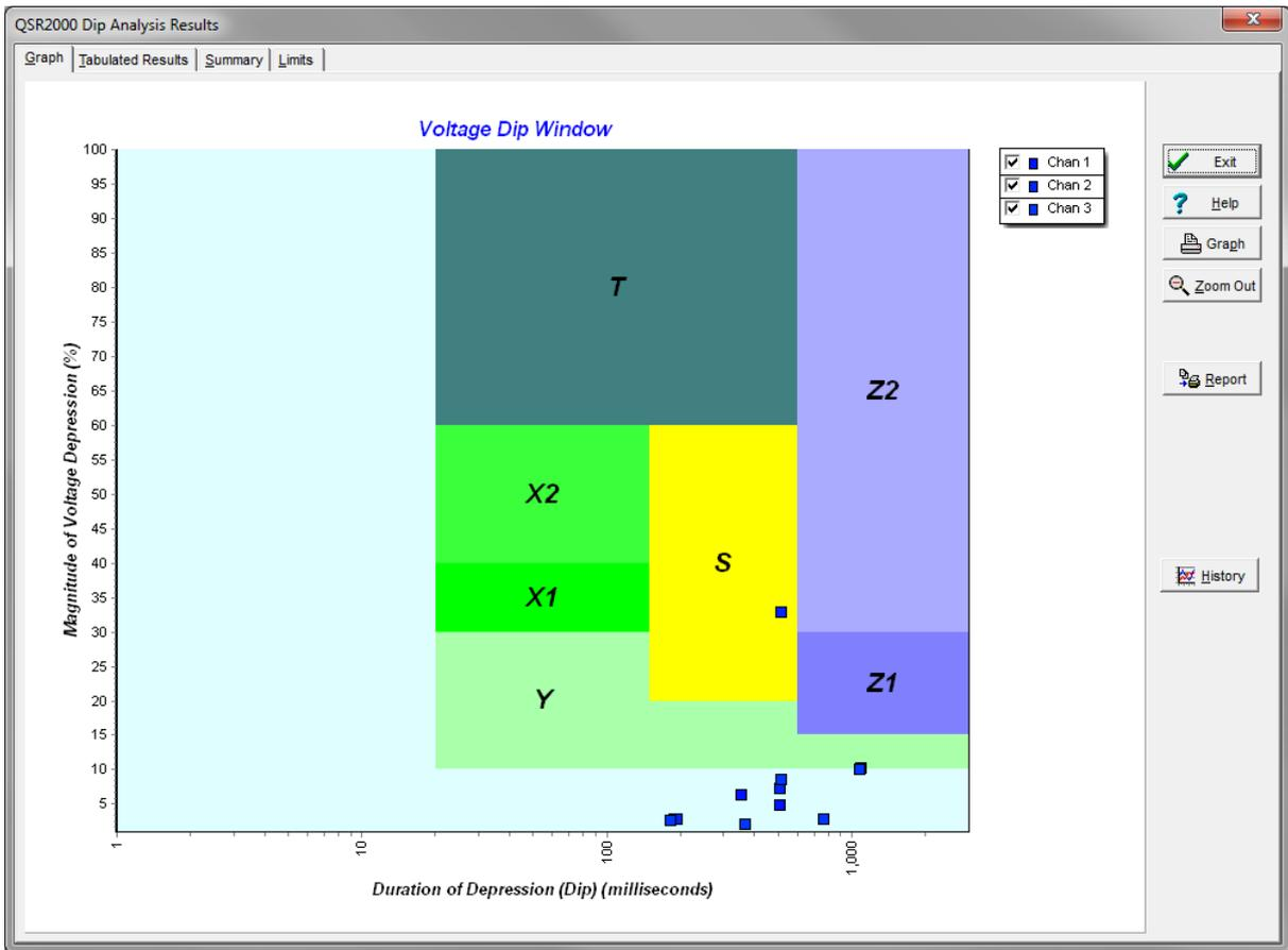
Fig. 12. 132kV substation supply disturbances – magnitude vs. duration.
