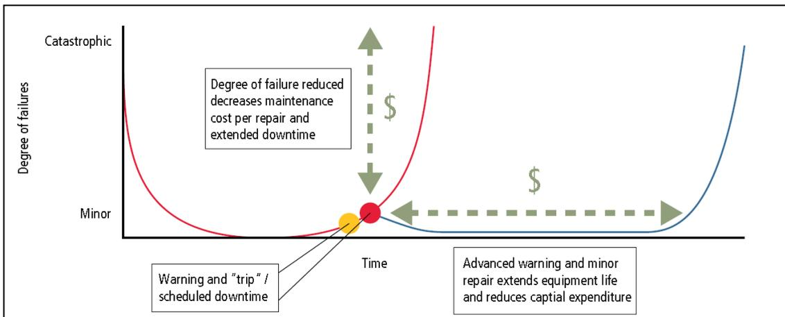
Fig. 2. Extending the bathtub curve with condition monitoring.
