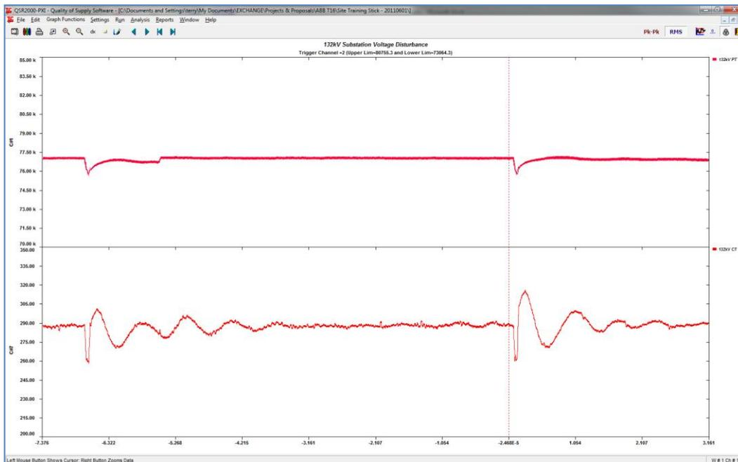
Fig. 10. Drive current (rms) response to multiple 132kV substation supply dips.
