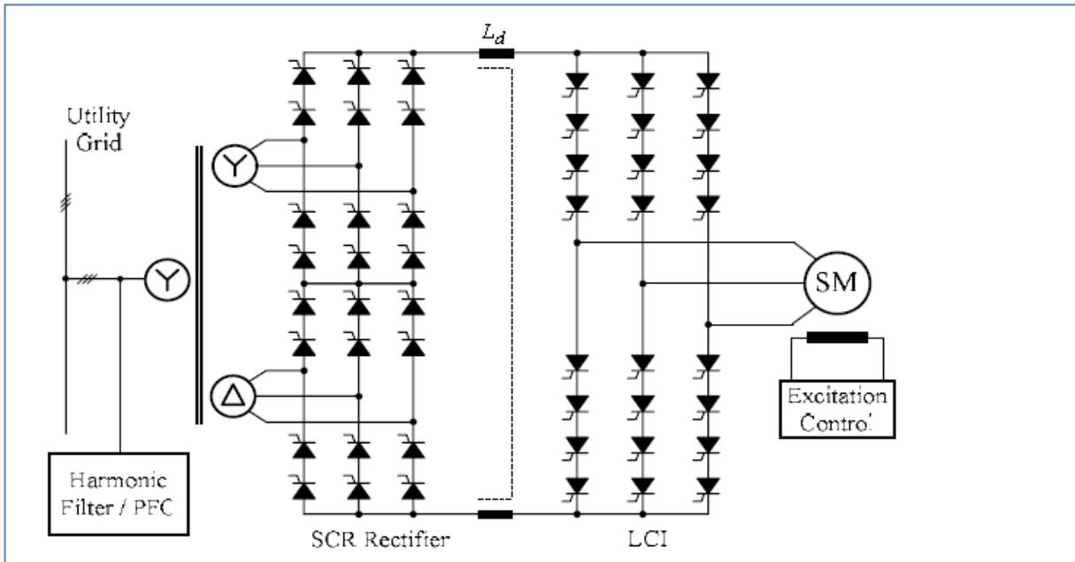
Fig. 5. Block diagram of a LCI fed synchronous motor.
