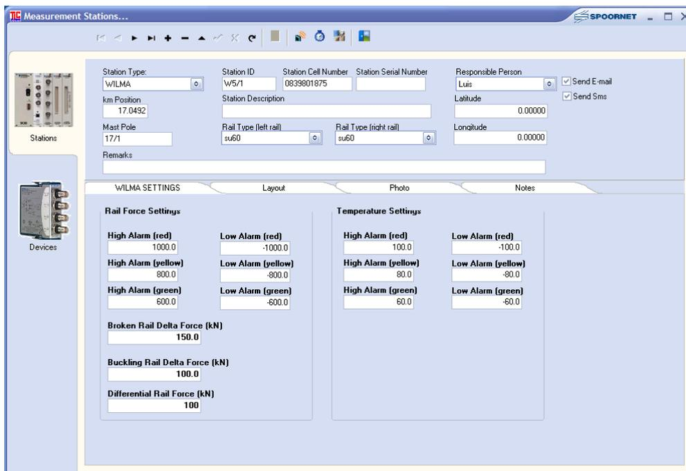
Fig. 16. Remote monitoring site configuration screen.
